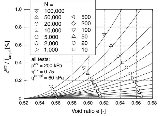
Figure 5. Determination of constant  $C_e$  by fitting of function  $f_e$
