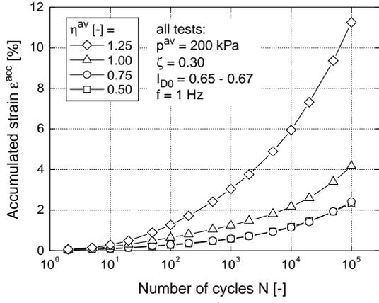
Figure 9. Accumulation curves in tests with different average stress ratios  $\eta^{av}$
