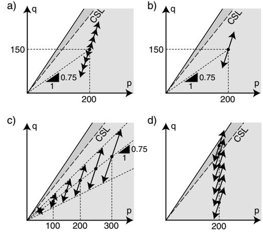
Figure 2. Suitable stress paths in the cyclic triaxial tests for the determination of the constants  $C_e$ ,  $C_p$ ,  $C_Y$ ,  $C_{N1}$ ,  $C_{N2}$ ,  $C_{N3}$  of the HCA model
