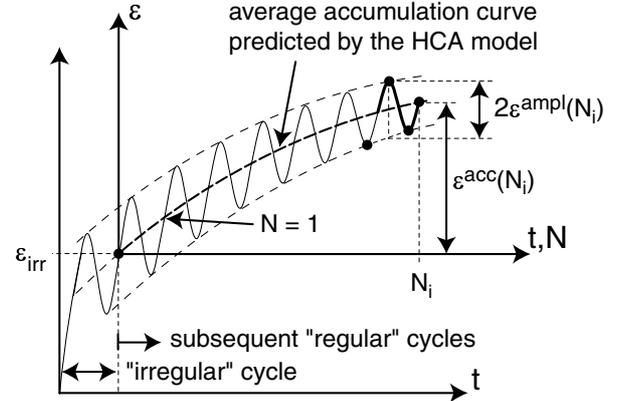
Figure 1. Typical curve  $\varepsilon(t)$  in a cyclic triaxial test
