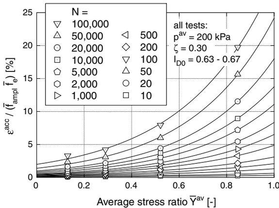
Figure 10. Determination of constant  $C_Y$  by fitting of function  $f_Y$
