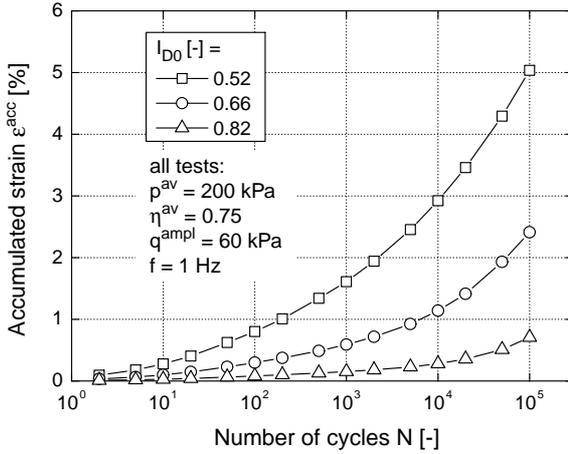
Figure 4. Accumulation curves in tests with different initial relative densities  $I_{D0}$
