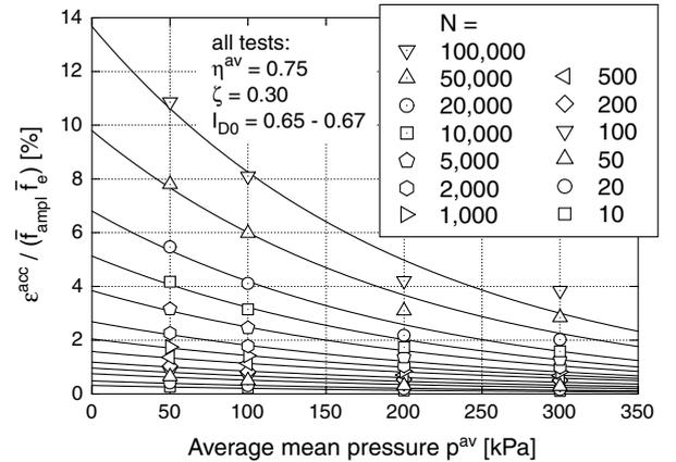
Figure 8. Determination of constant  $C_p$  by fitting of function  $f_p$
