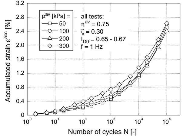
Figure 7. Accumulation curves in tests with different average mean pressures  $p^{\text{av}}$
