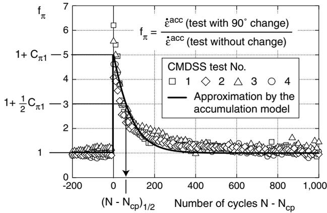
Figure 13. Decay of the increased accumulation rate during the cycles following the 90°-change of the polarization
