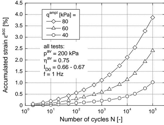
Figure 3. Accumulation curves  $\varepsilon^{\text{acc}}(N)$  in tests with different stress amplitudes  $q^{\text{ampl}}$
