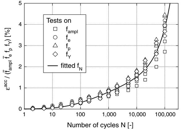
Figure 11. Fitting of function  $f_N$  to the data of all test series
