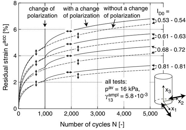
Figure 12. Temporary increase of the accumulation rate due to a sudden 90°-change of the polarization, results of cyclic multiaxial simple shear tests
