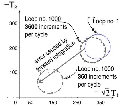
Figure 2: Accumulation of numerical error due to explicit (Euler forward) time integration. Theoretically no stress accumulation should be obtained in hyperelastic materials after a closed strain path. Euler backward integration causes an analogous error in the opposite direction.
