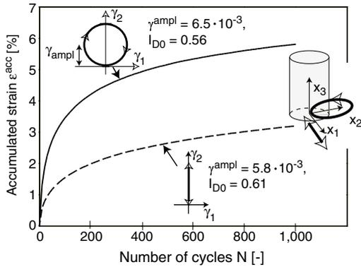
Figure 16: Circular strain loops generate approximately twice faster accumulation than the in-phase ones.
