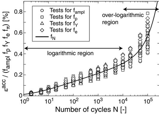
Figure 10: Accumulated strain  $\epsilon^{\text{acc}}$  divided by the functions  $f_{\text{ampl}}$ ,  $f_p$ ,  $f_\gamma$ ,  $f_e$  and  $f_\pi$  as a function of the number of cycles.
