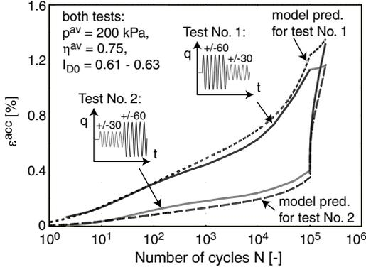
Figure 11: Numerical calculation and experimental verification of the Miner's rule.
