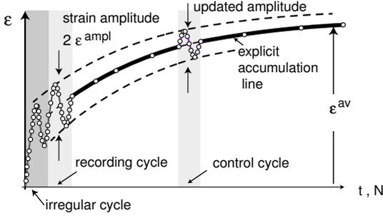
Figure 3: The basic idea of explicit calculation of the cumulative deformation.
