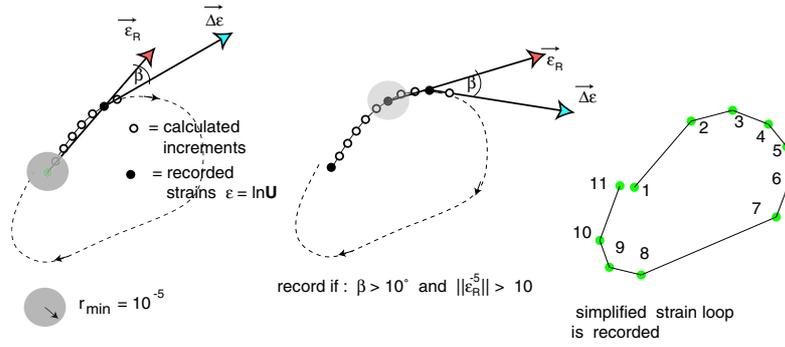
Figure 22: Recording of strain states along the loop.
