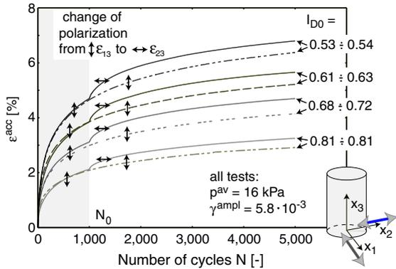
Figure 17: After a sudden change of polarization  $\vec{\mathbf{A}}_\varepsilon$  the rate of accumulation leaps.
