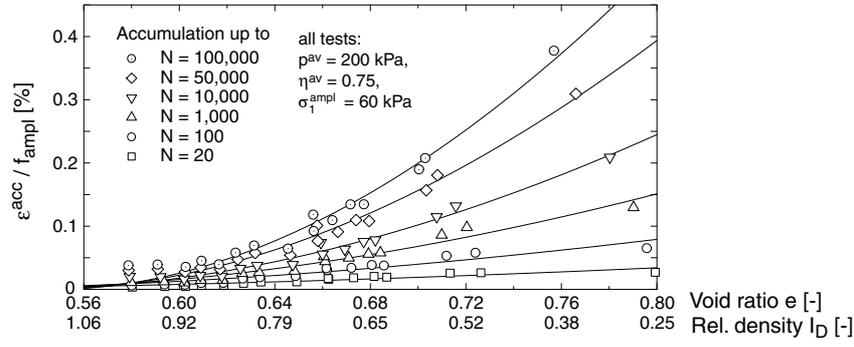
Figure 14: Accumulated strain  $\varepsilon^{\text{acc}}$  in dependence on the actual void ratio  $e$  for different numbers of cycles. The  $f_{\text{ampl}}$ -variability has been removed here.
