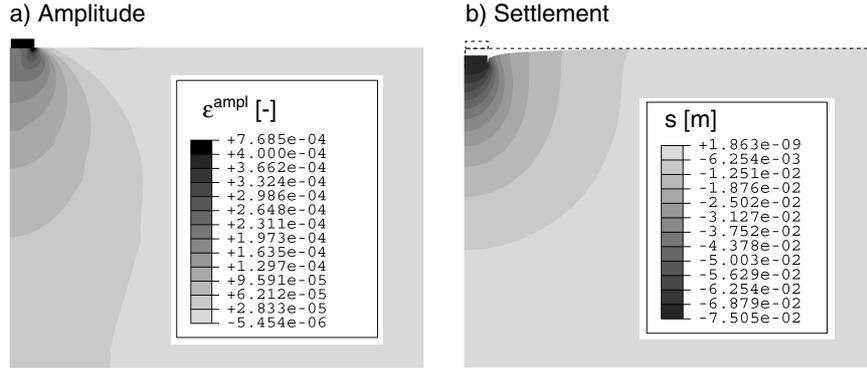
Figure 25: a) Field of strain amplitude  $\varepsilon^{\text{ampl}}$ , b) Field of accumulated settlement  $s^{\text{acc}}$  after  $N = 100,000$  cycles
