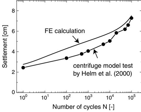
Figure 26: Accumulation of foundation settlement during the regular cycles: FE calculation versus model test.
