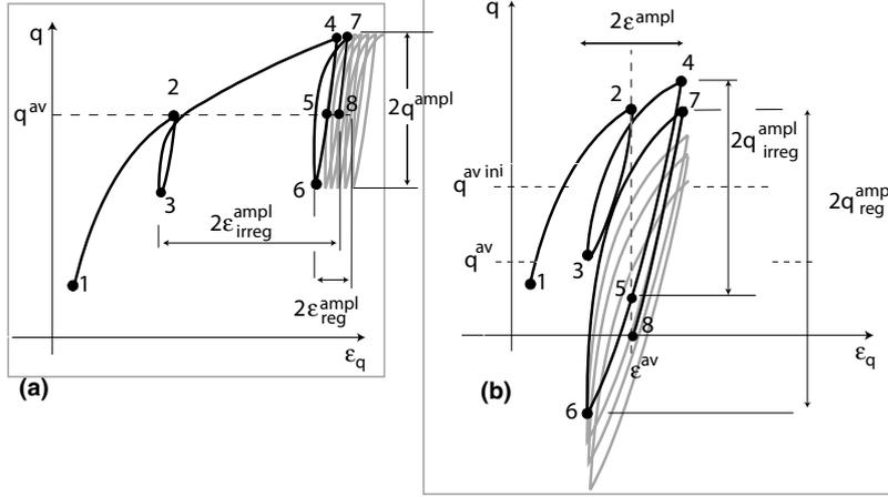
Figure 8: (a) Unsymmetric stress-controlled cycles. (b) Unsymmetric strain-controlled cycles. Monotonic loading 1-2 is followed by the irregular cycle (2-3-4-5) and the regular cycle (5-6-7-8). In the irregular stress-controlled cycle the strain amplitude  $\epsilon_{\text{irreg}}^{\text{ampl}}$  is too large. In the irregular strain-controlled cycle the stress amplitude is too small and, which is more important, the average stress changes from  $q^{\text{av ini}}$  to  $q^{\text{av}}$ .
