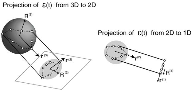
Figure 19: The directions  $\vec{r}_i$  and the sizes  $R^{(i)}$  of the strain loop.
