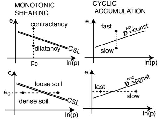
Figure 15: Lines of constant rate of accumulation in the  $e - \ln p$  diagram are differently inclined than the CSL. The notions 'loose' and 'dense' are pressure-dependent in the critical state soil mechanics. For cyclic accumulation this dependence is not analogous.
