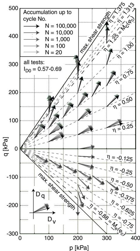
Figure 5: Directions  $\mathbf{m}$  of strain accumulation were determined from numerous cyclic triaxial tests for various stress ratios  $\eta^{\text{av}} = q^{\text{av}}/p^{\text{av}}$ . The initial index of density of a sample is denoted by  $I_{D_0}$ .
