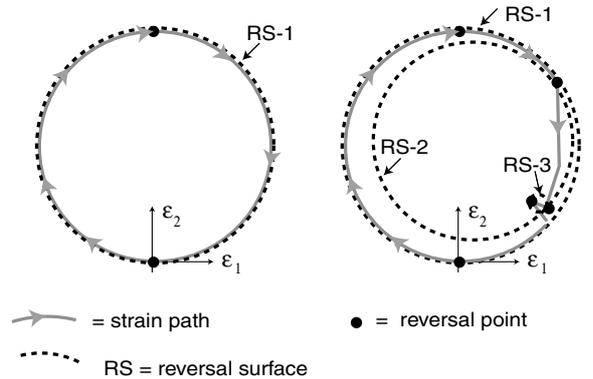
Figure 21: A multiaxial rainflow counting algorithm has a short-coming: a relatively small modification of the strain path generates the reversal surface RS-2 of a considerable size. RS-2 is counted as a sub-cycle.
