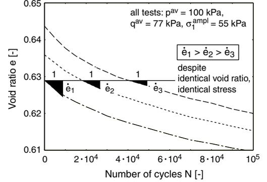
Figure 9: The effect of cyclic loading history on the rate of densification  $\dot{e} = de/dN$  measured during cyclic drained triaxial test.
