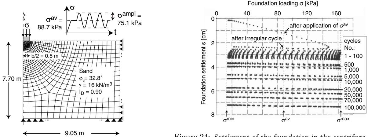
Figure 23: Geometry of the prototype and soil parameters of the centrifuge test.
