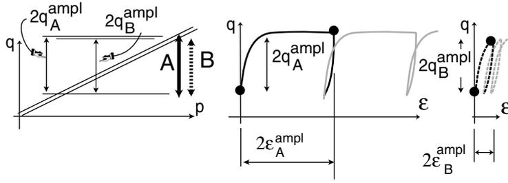
Figure 7: Unsymmetric stress-controlled cycles. The large cycles A (solid line) which encounter the yield surface (double line) are poorly described by the stress amplitude  $q_A^{\text{ampl}}$  alone. The stress path B (dotted line) which approaches only the yield surface without touching it has almost the same stress amplitude  $q_B^{\text{ampl}} \approx q_A^{\text{ampl}}$  but the respective strain amplitudes are quite different and so are the rates of accumulation.
