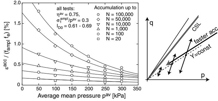
Figure 13: Accumulated strain  $\epsilon^{\text{acc}}$  in dependence on the average mean pressure  $p^{\text{av}}$  for different numbers of cycles. The diagrams have been purified from the variability of  $f_{\text{ampl}}$  and  $f_e$ .
