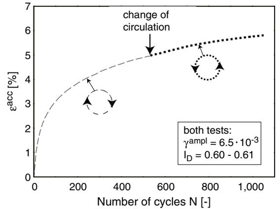
Figure 18: A change of the circulation of the cyclic strain path does not affect the accumulation.
