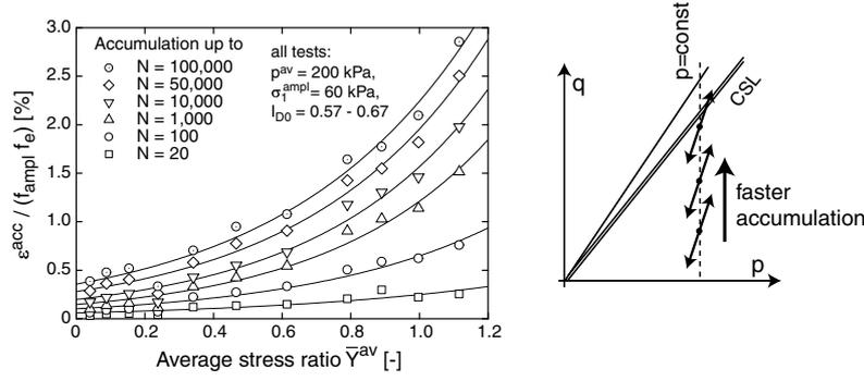
Figure 12: Accumulated strain  $\epsilon^{\text{acc}}$  as a function of the average stress ratio  $\bar{Y}^{\text{av}}$  for different numbers of cycles. The diagrams have been purified from the variability of  $f_{\text{ampl}}$  and  $f_e$ .
