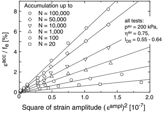
Figure 6: The rate of accumulation is proportional to the square of the strain amplitude. The diagram has been purified from the variability of  $f_e$ .
