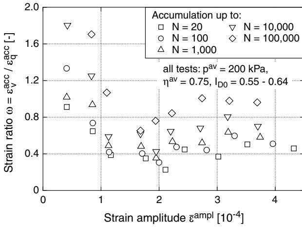
Fig. 9: Strain ratio  $\omega$  as a function of the strain amplitude  $\varepsilon_v^{\text{ampl}}$
