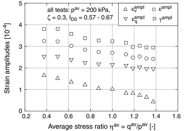
Fig. 15: Strain amplitudes in tests with different average stress ratios  $\eta^{\text{av}}$  (mean values during  $10^5$  cycles)
