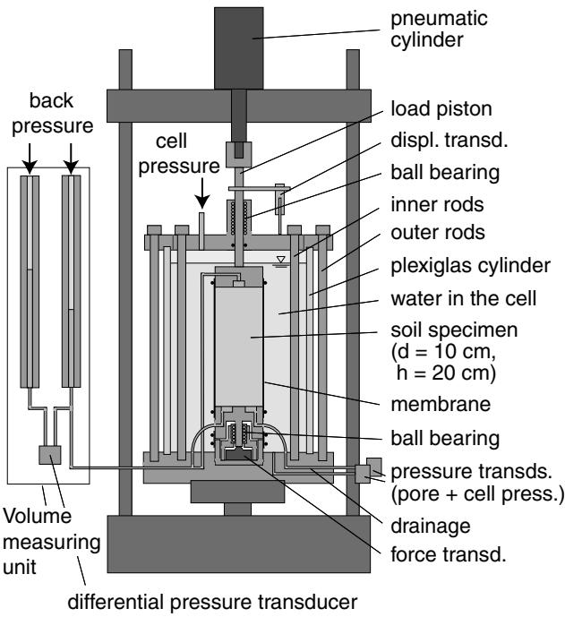
Fig. 3: Scheme of cyclic triaxial test device
