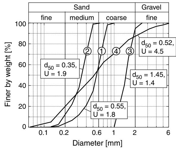
Fig. 4: Tested grain size distribution curves ( $d_{50}$ : mean grain diameter,  $U = d_{60}/d_{10}$ : uniformity index)
