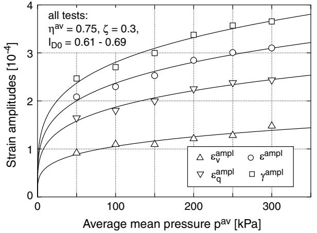
Fig. 11: Strain amplitudes in tests with different average mean pressures  $p^{\text{av}}$  but  $\zeta = \text{const}$  (mean values during  $10^5$  cycles)
