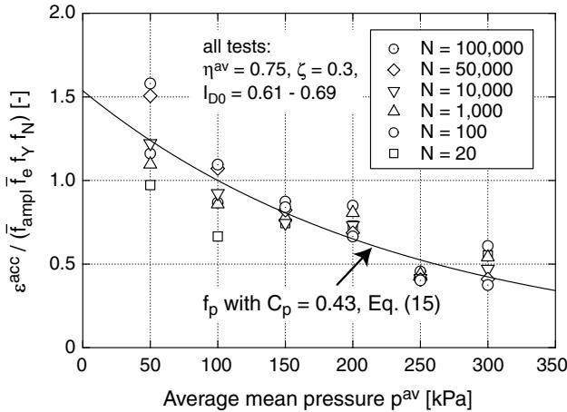
Fig. 13: Accumulated strain  $\varepsilon^{\text{acc}} / (\bar{f}_{\text{ampl}} \bar{f}_e \bar{f}_Y \bar{f}_N)$  in dependence on the average mean pressure  $p^{\text{av}}$
