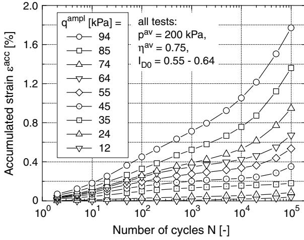
Fig. 6: Accumulation curves  $\varepsilon^{\text{acc}}(N)$  in tests with different stress amplitudes  $q^{\text{ampl}}$
