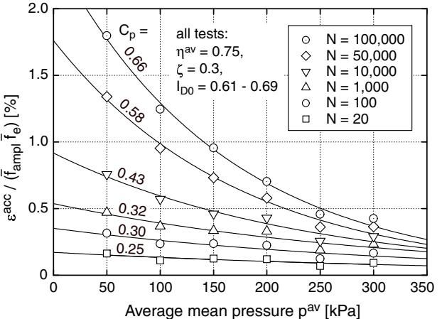
Fig. 12: Accumulated strain  $\varepsilon^{\text{acc}} / (\bar{f}_{\text{ampl}} \bar{f}_e) [\%]$  in dependence on the average mean pressure  $p^{\text{av}}$
