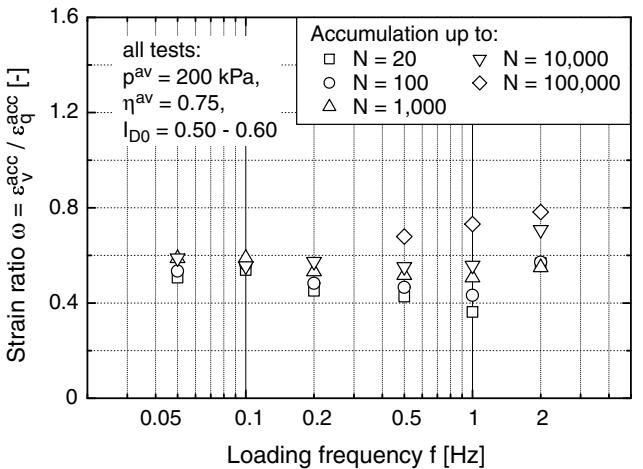
Fig. 27: Strain ratio  $\omega$  versus loading frequency  $f$
