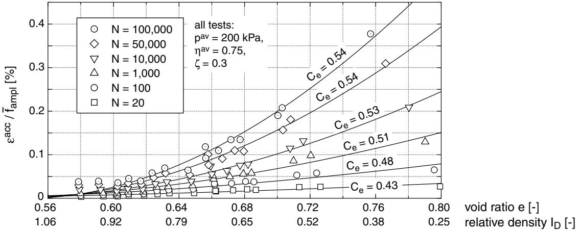
Fig. 22: Accumulated strain  $\varepsilon^{acc}/\bar{f}_{ampl}$  in dependence on the void ratio  $e$  or the relative density index  $I_D$ , respectively
