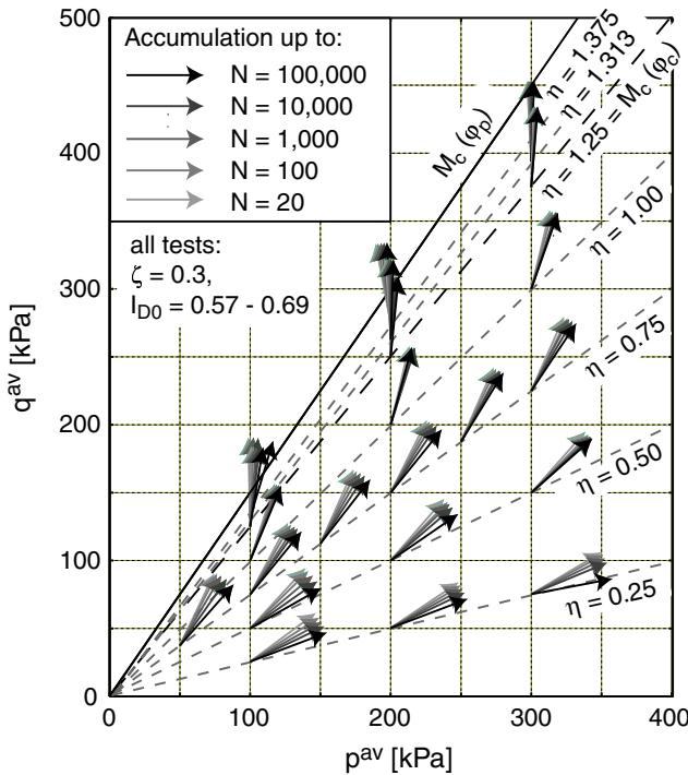
Fig. 20: Direction of accumulation in the  $p$ - $q$ -plane for different average stresses
