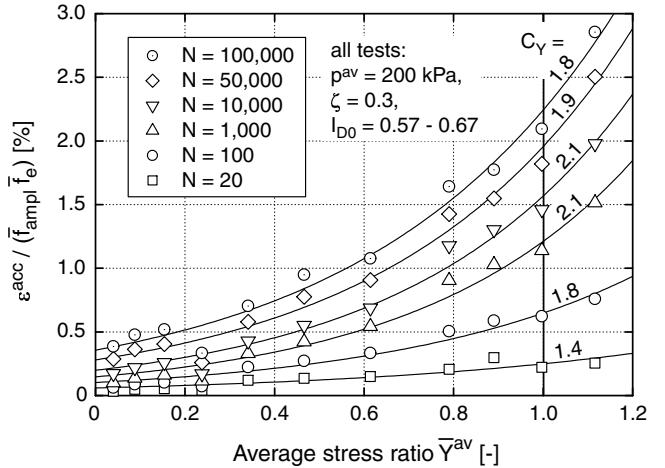
Fig. 16: Accumulated strain  $\varepsilon^{\text{acc}} / (\bar{f}_{\text{ampl}} \bar{f}_e)$  in dependence on the average stress ratio  $\bar{Y}^{\text{av}}$
