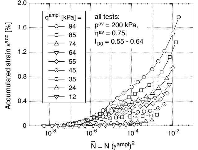
Fig. 8: Accumulated strain  $\varepsilon^{\text{acc}}$  in dependence on  $\tilde{N} = N (\gamma^{\text{ampl}})^2$  as proposed by Sawicki and Świdziński [12,13]
