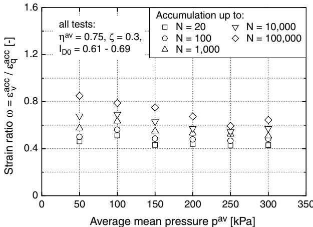
Fig. 14: Strain ratio  $\omega$  as a function of the average mean pressure  $p^{\text{av}}$
