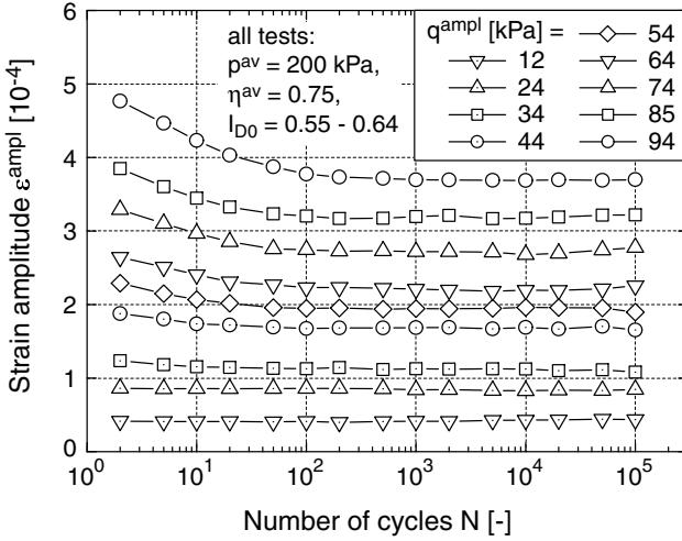
Fig. 5: Strain amplitude  $\varepsilon^{\text{ampl}}$  versus the number of cycles  $N$
