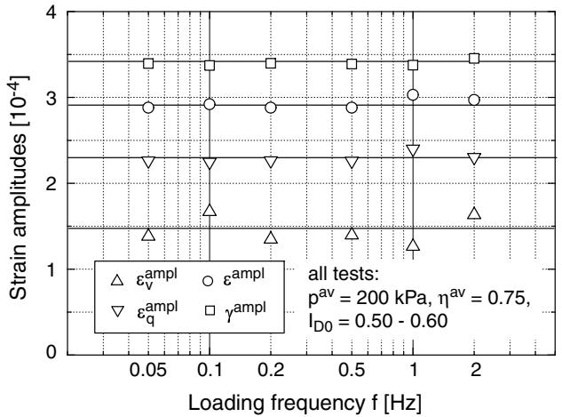
Fig. 25: Strain amplitudes as a function of the loading frequency  $f$
