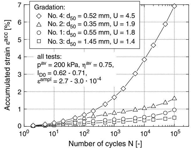
Fig. 29: Accumulation curves  $\varepsilon^{\text{acc}}(N)$  for different gradations
