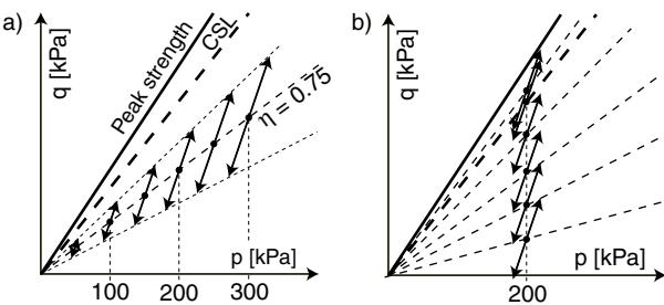
Fig. 10: Stress paths in tests on the influence of the average stress, a) variation of  $p^{\text{av}}$ , b) variation of  $\eta^{\text{av}}$
