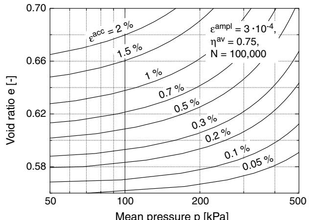
Fig. 23: Curves of identical accumulation in the  $e$ - $\ln(p)$ -diagram
