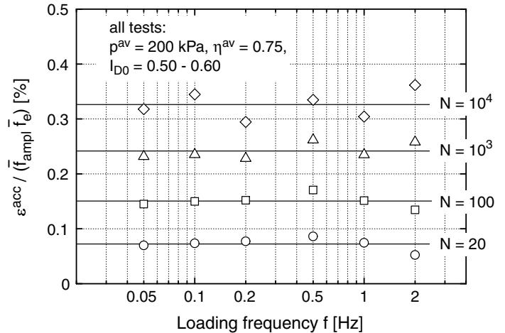
Fig. 26: Residual strain  $\varepsilon^{\text{acc}} / (\bar{f}_{\text{ampl}} \bar{f}_e)$  for different loading frequencies  $f$
