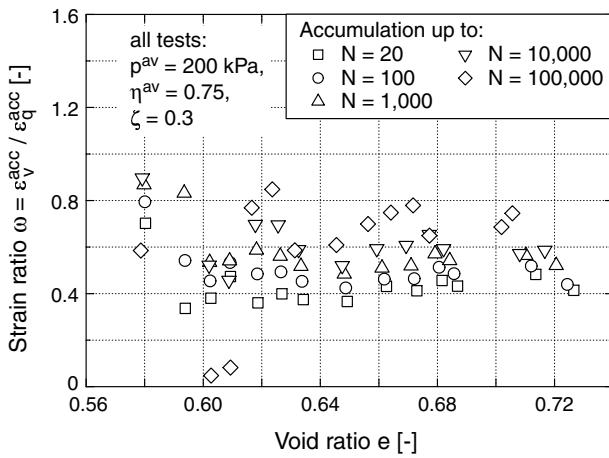
Fig. 24: Strain ratio  $\omega$  as a function of the void ratio  $e$
