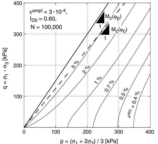
Fig. 19: Curves of identical accumulation in the  $p$ - $q$ -plane
