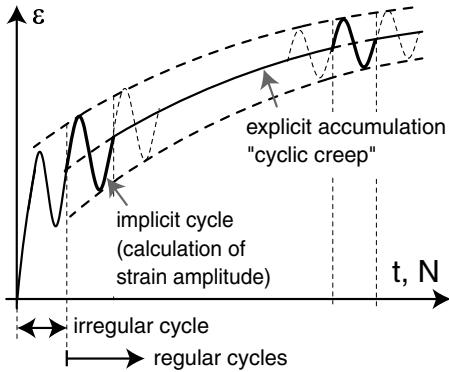
Fig. 1: Calculation procedure of explicit models
