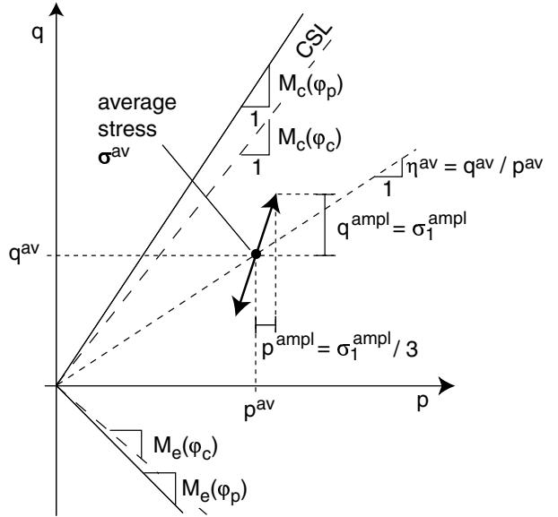
Fig. 2: State of stress in a cyclic triaxial test
