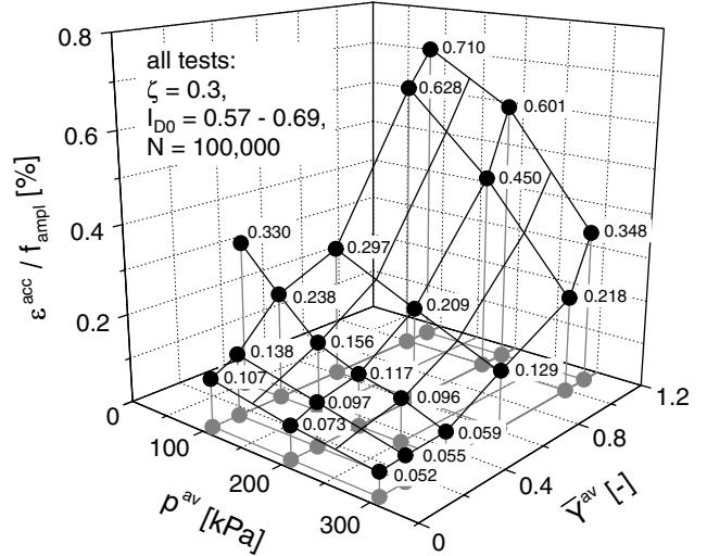
Fig. 18: Accumulated strain  $\varepsilon^{\text{acc}}$  after 100,000 load cycles for different average stresses  $\sigma^{\text{av}}$
