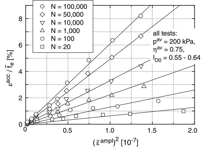
Fig. 7: Accumulated strain  $\varepsilon^{\text{acc}}/\bar{f}_e$  as a function of the square of the strain amplitude  $(\bar{\varepsilon}^{\text{ampl}})^2$
