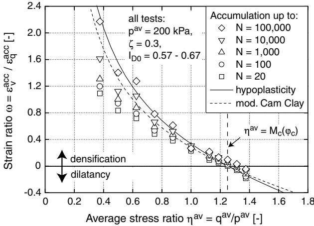
Fig. 17: Strain ratio  $\omega$  as a function of average stress ratio  $\eta^{\text{av}}$
