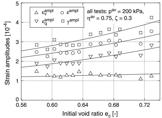
Fig. 21: Strain amplitudes in tests with different initial void ratios  $e_0$  (mean values during  $10^5$  cycles)
